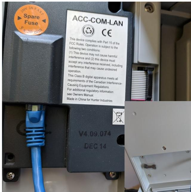
Connect ACC-COM-LAN module to Ethernet network using standard networking equipment – patch cables, switches etc.
